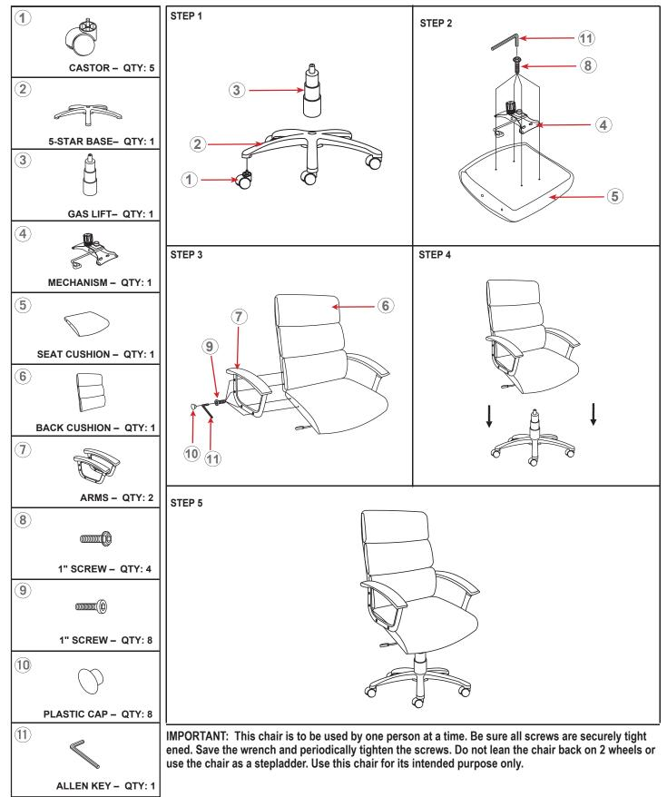
**PARTS** – remove all the parts from the carton and verify part quantities as indicated on this parts list.
