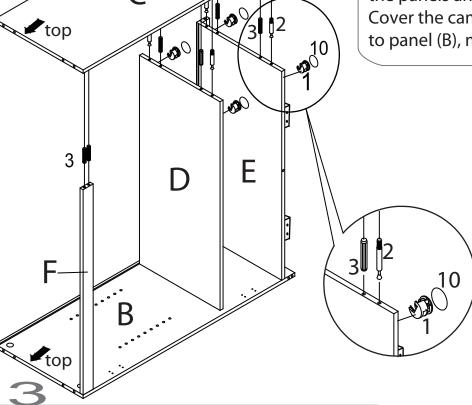
Attach the cam bolts (2) and the wood dowels (3) on panels (C) in the areas illustrated. Then insert the cam locks (1) into panels (D) and (E) with the arrows on the cam locks facing the holes to the side of the panels (D & E). Attach the panels and secure the cam locks, turning clockwise to lock. Cover the cam locks with the adhesive covers (10).
