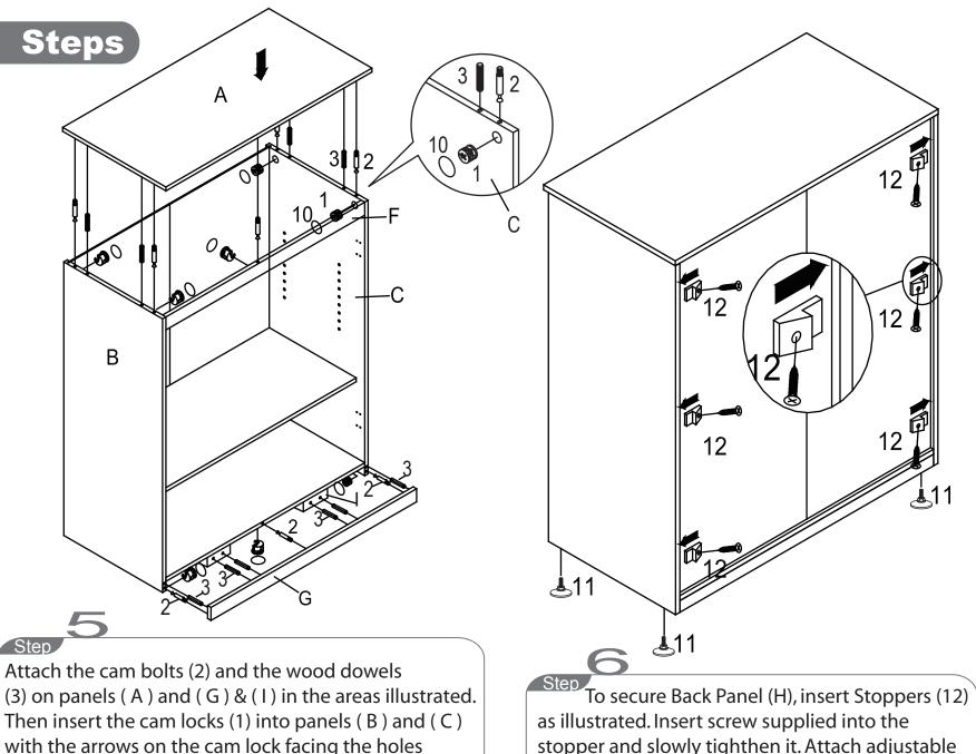
(3) on panels (A) and (G) & (I) in the areas illustrated. Then insert the cam locks (1) into panels (B) and (C) with the arrows on the cam lock facing the holes to the side of the panels. Attach the panels and secure the cam locks, turning clockwise to lock. Cover the cam locks with the Adhesive covers (10).
