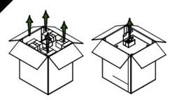
Remove the corner protectors, open the box that contains the casters B C and remove.
