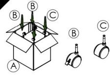
Twist the back caster © and front caster with brake B into main body A plate as shown. Place fifth craster D in the middle front of the main body
