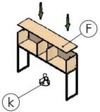
Place the cover(F) on top of the estructure and secure with glides 12 mm(k).
