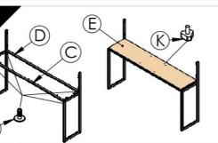
Assemble the support bars (C) and (D) with left and right leg (A) (B) joining them with screws 15 mm, (M) Place the base and secure with srews 15 mm (M) and glides 12 mm(K).
