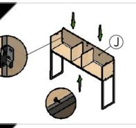
Assemble back side (J) with right and letf sides joining them with the hooks
