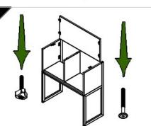
Put the sides  $\bigcirc$  on left and right legs  $\bigcirc$  B tighten the vise  $\bigcirc$  , put the division  $\bigcirc$  with the glide  $\bigcirc$  , hook the back side  $\bigcirc$  to sides  $\bigcirc$  D.
