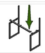
Put the support bar  $\bigcirc$  into left leg and right leg  $\bigcirc$   $\bigcirc$   $\bigcirc$   $\bigcirc$  into left leg and right leg  $\bigcirc$   $\bigcirc$   $\bigcirc$   $\bigcirc$  into left leg and right leg  $\bigcirc$   $\bigcirc$  into left leg and right leg  $\bigcirc$  into left leg and right leg and
