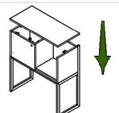
Attach the door (H) to the side (F), Put the cover (E) on the top and tighten the glides (I).
