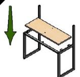
Put the base  $\bigcirc$  over left leg and right leg  $\bigcirc$   $\bigcirc$  , tighten the glides  $\bigcirc$  at the base to the legs.
