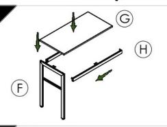
Hook the return support bar  $\widehat{\mathbb{H}}$  to the return leg  $\widehat{\mathbb{F}}$  then place top the return cover  $\widehat{\mathbb{G}}$  to return support bar, tighten knobs of 12mm  $\widehat{\mathbb{L}}$  to connect top cover to the legs.
