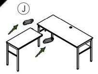
Hook the return support bar (H) to the support bar (E), place the union plate (J) joining return with cover, tighten knobs of 12mm (T) to connect the desk to the return.
