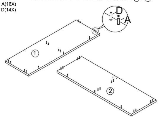
9. INSTALL "B" KLIX CAMS INTO PANELS ③ 4 5 7 & 8 .CONNECT PANEL 1 TO 3 4 5 & 7 USING INSTALLED "A" CAM SCREWS AND "D" DOWELS, TIGHTEN. REPEAT TO CONNECT PANEL 2 TO 3 4 5 & 8 .
