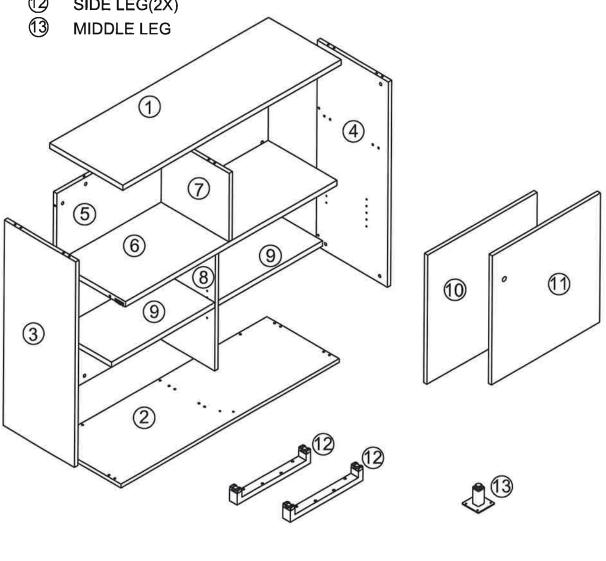
1. INSTALL "A" CAM SCREWS AND "D" DOWELS TO UNDERSIDE OF PANEL®, INSTALL "B" KLIX CAMS INTO PANEL ®. THEN CONNECT®TO PANEL® ,TIGHTEN. A(2X) B(2X) D(2X)
