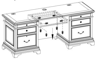
Attach Typical Swivel Keyboard to Mounting Plate by using 4 bolts, lock washers, flat washers and nuts. Use hex wrench to tighten all these bolts. (These hardware attached with Keyboard)
