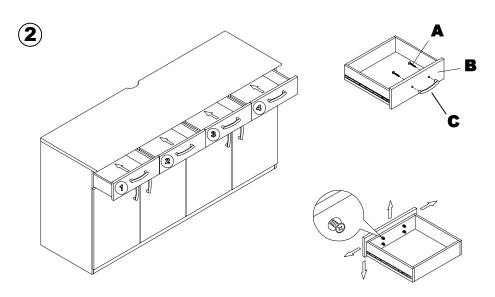
Drawer face alignment. If the drawer front panels are mis-aligned you can adjust them by loosening the four (4) screws on the inside of the panel. Move the panel into the correct location and re-tighten the screws.
