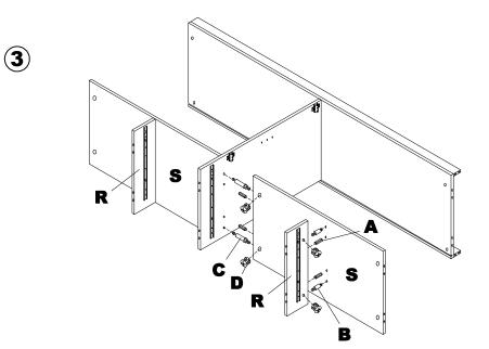
Note: For Step 3, dowels (A) are to be inserted into drawer support (R) and edge of dividers (S), NOT in face of divider (S) or center support (P).
