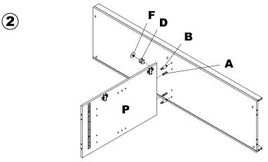
Note: For Step 2, dowels (A) are to be inserted into center support (P) and NOT into bottom panel (N).
