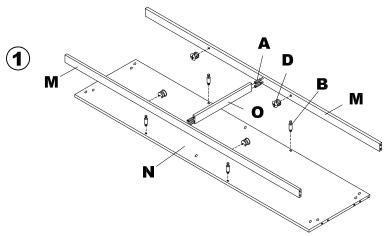
Note: For Step 1, dowels (A) are to be inserted into brace (O) and NOT into toe kick (M).
