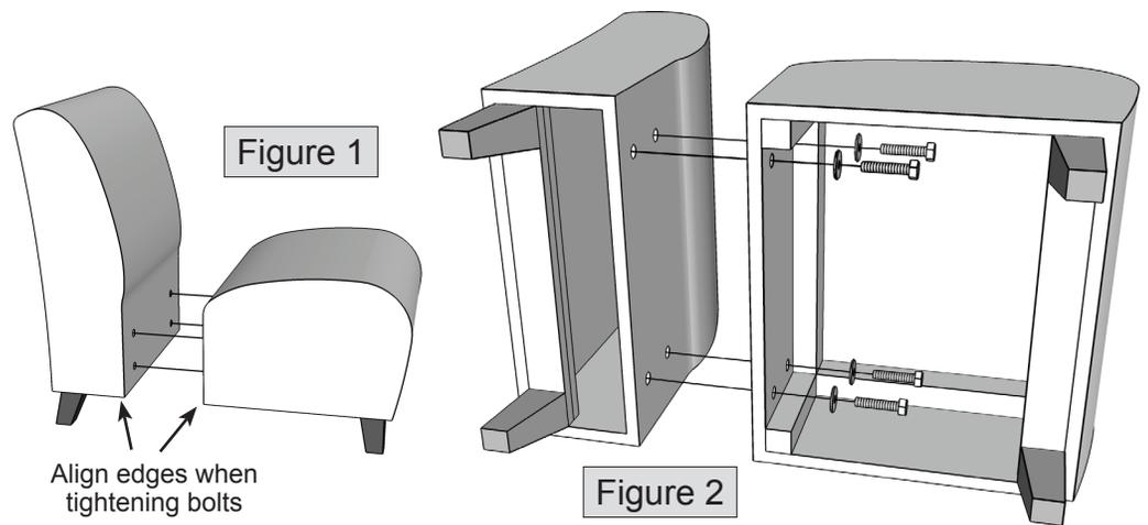
1. Follow instructions in Section 1 to attach seat to back. Align bottom edge of seat with bottom edge of back and tighten bolts securely.
