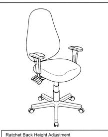
Ratchet Back Height Adjustment To raise the back, slowly lift the back up until you hear a series of 4 to 5 clicks. Each click represents a position where the back will lock into place. To lower the back, raise the back all the way up until tension is released - the back will then return to the lowest position without stopping. Raise back up to desired position.
