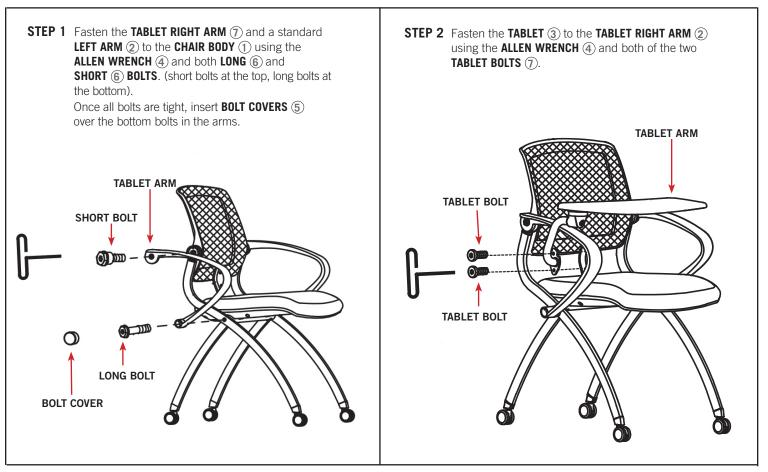
TIP: Do not tighten bolts one at a time. Instead, tighten each a little, alternating a few turns at a time until all are tight..
