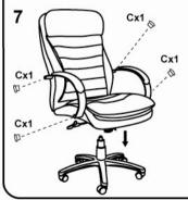
Note: Please tighten all arm screws using allen key before step 7
