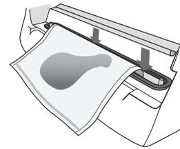
5. Lower Bar, press Vacuum & Seal button (Fig. 4).
