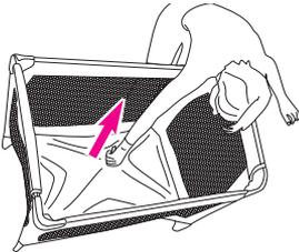
**DO NOT** unlock top rails yet. Center of floor must be halfway up before top rails will unlock.
