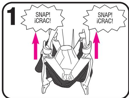
1. Pull up on all 4 sides and snap into place. Do not push center of Playard down until top rails are locked. (See pages 7 and 8)
