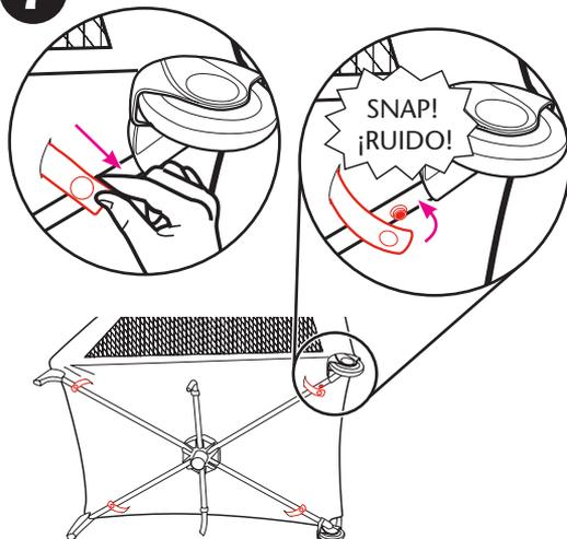
Pull strap through bottom of playard and wrap around tube and refasten snap. Repeat on other corners.
