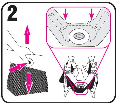
2. Lift rail up slightly, press button and lower rail. Repeat on all 4 sides. (See page 10 and 11)
