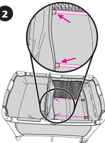
Insert mattress support tubes to tube tunnels.
