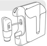
To attach Bag Holder, align the tabs on the holder above the tabs on the appliance and push holder downward to lock holder on the appliance.
