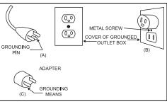
This heater is for use on 120 volts. The cord has a plug as shown in the figure below. An adapter as shown at C is available for connecting three-blade grounding-type plugs to two-slot receptacles. The areen arounding lug extending from the adapter must be connected to a permanent ground such as a properly grounded outlet box. The adapter should not be used if a three-slot grounded receptacle is available.
