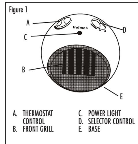
3. The Power Light will remain lit during operation, until the unit is unplugged.
