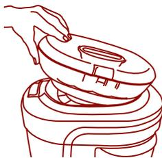
**NOTE: IF ICE RESERVOIR IS NOT SEATED FIRMLY IN PLACE THE UNIT WILL NOT OPERATE.**
