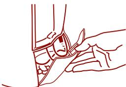
4. Remove the Ice Reservoir Lid using the Release Button located on the top of the Ice Reservoir.
