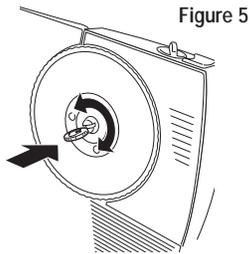
The Blade should not be left to soak in water. Wash, rinse, and dry Blade immediately. Install Blade in main unit after it has dried.
