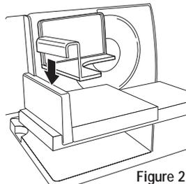
NOTE: It is important to always return the Thickness Adjustment Knob to setting '0'. The Feeder should be placed in the locked position after use.
