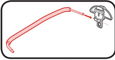
4. Insert the long end of the tube into the button housing as shown.
