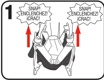
1. Pull up on all 4 sides and snap into place. Do not push center of Playard down until top rails are locked. (See pages 8 and 9)
