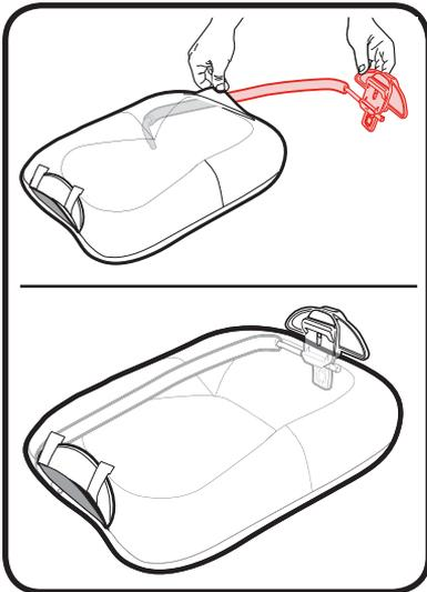
6. With the seat side up, insert the button housing tube as shown.
