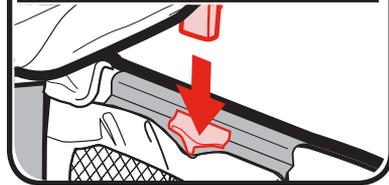
12. The tabs on the sides of the seat will snap in place as shown.
