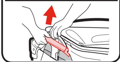
2. Press button and pull up on seat/changer to release. Repeat steps 1- 2 on the opposite side.
