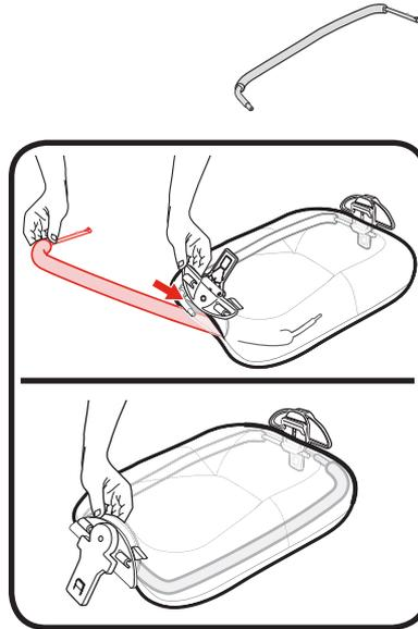
8. Insert the button housing tube as shown. The metal button should be facing out when snapped in place as shown.
