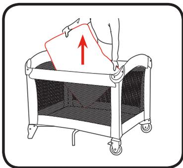
2. **DO NOT** unlock top rails yet. Pull the center of the playard floor up with the tab in the middle of the playard. Center of floor must be halfway up before top rails will unlock.
