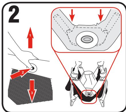
2. Lift rail up slightly, press button and lower rail. Repeat on all 4 sides. (See page 16)
