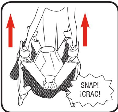
3. Pull up on side rails in middle above push button until all four sides are locked. **DO NOT** push center down yet.
