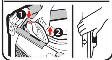
2. Push down on the inside of changer until it clicks into place. **Check** that changer is securely attached by pulling up on it.
