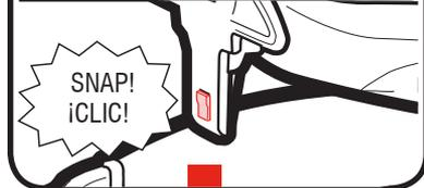
13. Push down on the inside of seat/changer until it clicks into place. Check that seat/changer is securely attached by pulling up on it.
