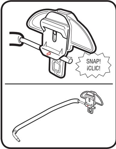
5. The metal button should be facing out when snapped in place as shown.
