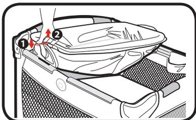
1. Press button ❶ and pull up ❷ to unlock and rotate to the seat side.
