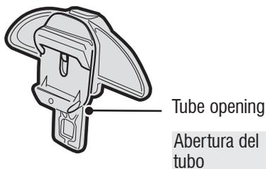
1. Press button ❶ and pull up ❷ to unlock and rotate as shown.
