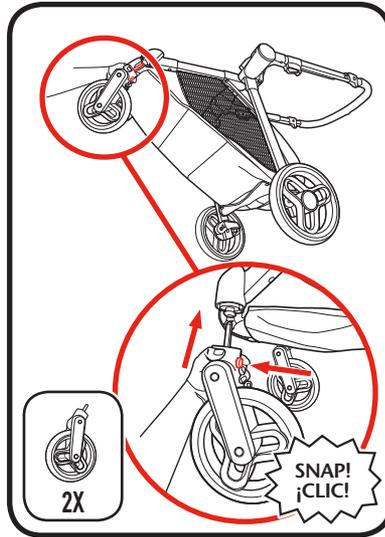
2. **CHECK** that wheels are securely attached by pulling on wheel assembly.
