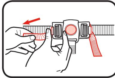
6. To open, press button on buckle to release the waist straps.
