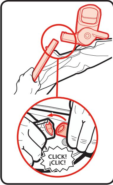
1. Attach lower seat frame tubes as shown.
