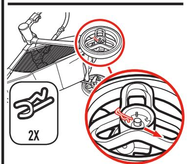
3. Push straight side of pin through axle hole. Pin will separate around the axle. Curved end of pin **MUST** face out as shown. Repeat on other end.
