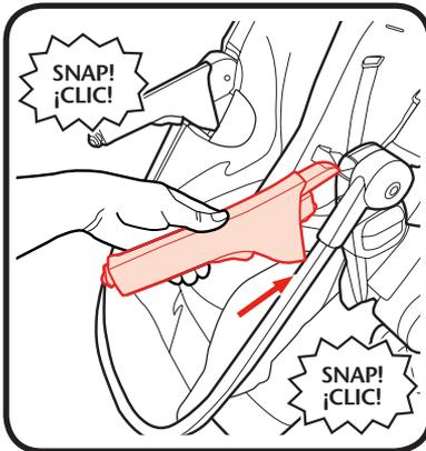
1. Insert armrests into slots on each side of the stroller until they click into place.
