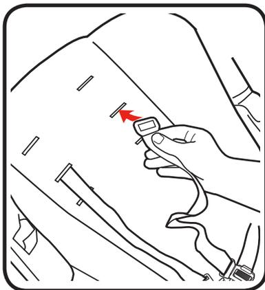
Push harness anchor through the front of the seat then re-insert through desired slots at the same height level. Use slide adjuster for further adjustment.
