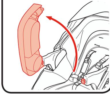
4. To remove child's tray, press buttons on bottom of both ends, and lift off.
