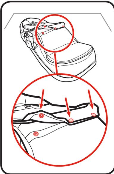
2. On the back of the seat, secure flap around seat wire with 3 snaps.
