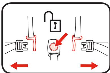
1. To open, press button on buckle to release the waist straps.
