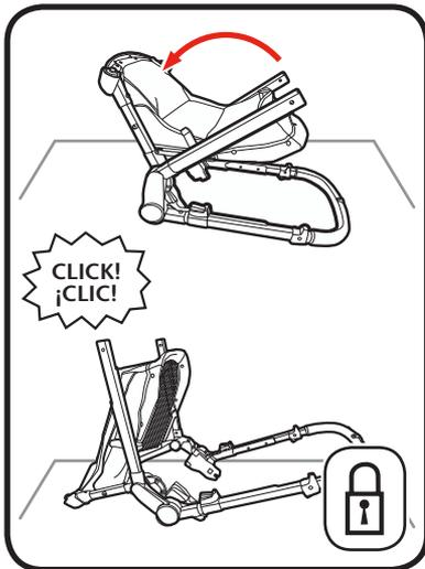
2. Lift basket of stroller up. **CHECK** that the stroller is completely latched open every time you open the stroller and before continuing with the rest of the assembly steps.
