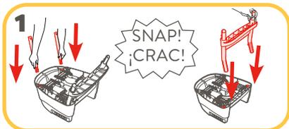
Flip seat base over, insert angled top rear legs and foot rest legs into leg mounts in seat as shown.
