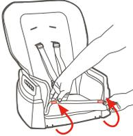
Disconnect elastic from bottom of seat base as shown.
