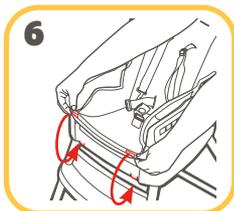
Attach elastic to hooks on bottom of seat base as shown.
