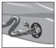
Remove nozzle of hose from inflation end and attach to opposite deflation end of pump. Repeat same steps as inflation. This will draw the air out quickly.
