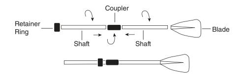
The assembled oar is to be inserted into the oar locks from the outside of the product. The oar retainer ring is then placed onto the top half of the assembled oar, from the inside of the product, to prevent the oar from sliding into the water (see below).
