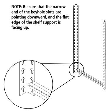
**3.** Assemble another unit end by repeating the directions in step 2. Be sure the shelf support rivets are seated in the bottom of the slots. If you are creating a starter unit and adder units then you will need to replace the EUR upright post on one end with ZTP upright posts.
