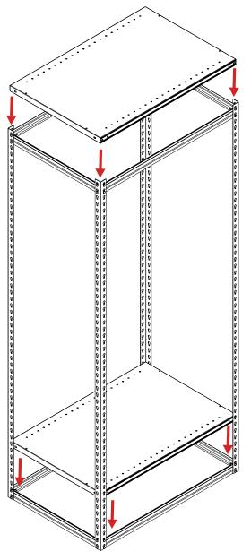
7. Next attach the ZSC-1 shelf clips (Ref. No. 6) to the EUR post as shown. Make sure that all four clips are on the same level on each of the uprights for the shelves to be level. Be sure to drive the clips down until they are seated firmly then install the shelf on top of the four clips, with the shelf sliding into the slot in the clip.
