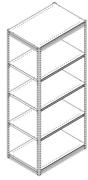
**9.** If you are assembling an adder unit it will not look like the drawing above. The adder unit will share front and back supports with the starter unit on the side that the starter unit is connected using an intermediate "T" post. To attach an adder unit to a starter unit you will attach the VDRS supports to the ZTP post and construct the adder unit the same way that you did the starter unit.
