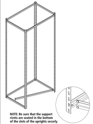
**6.** After building the framework, place a steel shelf (Ref. No. 5) on the lower level and on the top level of the VDRS supports. These shelves will lay directly on the flat ledge of the support.
