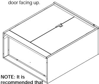
the bottom of the cabinet is a minimum of 1/2" off the floor, in order to more easily attach the caster kit to the unit.
