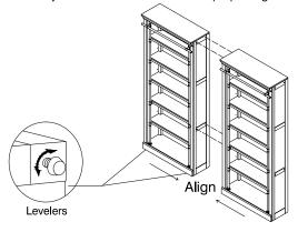
4 Using the provided Allen wrench (C) lightly screw bolts through the interior of the each cabinet. Once all bolts are in place, tighten to secure in place.
