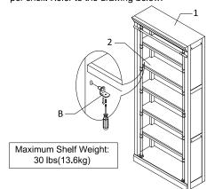
2 Anti-tip hardware kit must always be used to prevent the console
