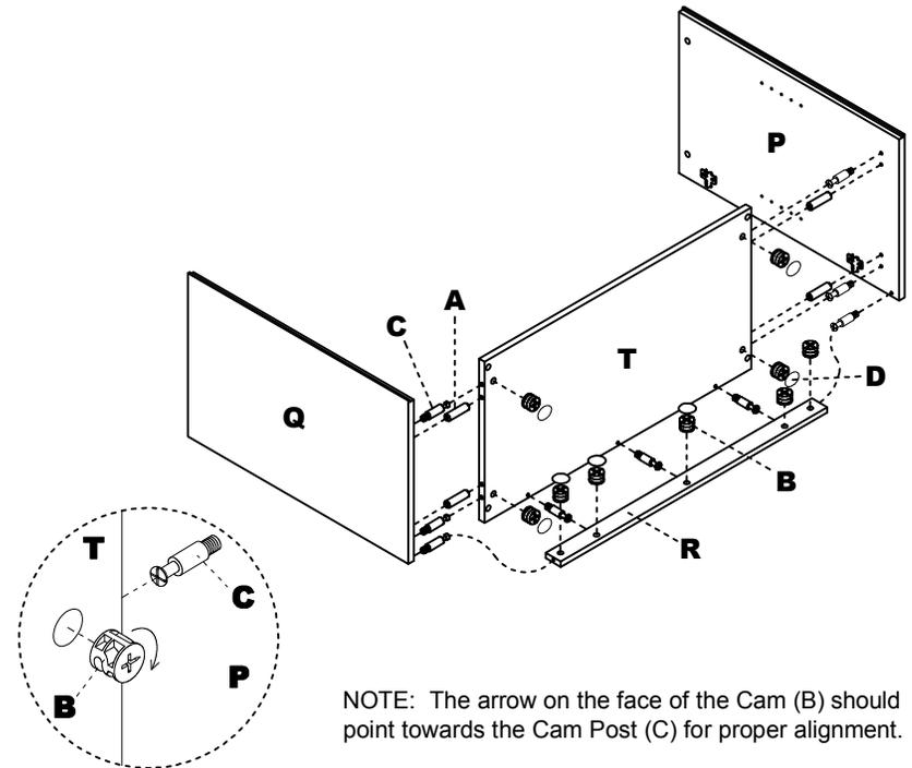
NOTE: The arrow on the face of the Cam (B) should point towards the Cam Post (C) for proper alignment.
