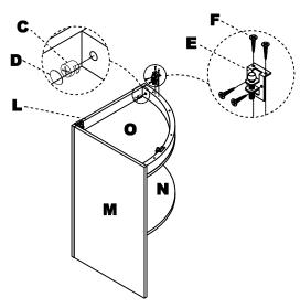
Attach Top (K) to Side Panels (L & M) by turning Cams (C). Apply Cam Stickers (D) onto Cams (C) of Side Panels (L & M).
