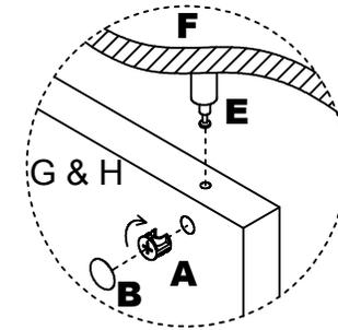
NOTE: The arrow on the face of the Cam (A) should point towards the Base Stand-off (E) for proper alignment.
