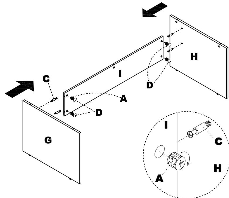
NOTE: The arrow on the face of the Cam (A) should point towards the Cam Post (C) for proper alignment.
