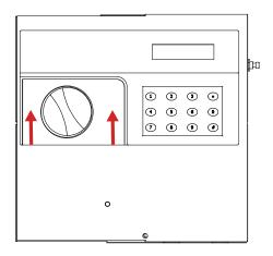
2. Remove the cover by prying it up from the bottom.
