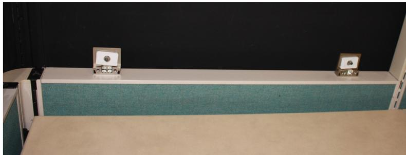
9. Take the mullion and line up the holes with the pegs on either PGHM. Then place the mullion onto the PGHM pegs.
