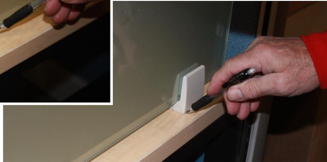
2. Worksurface does not have the holes drilled upon arrival. To start, put PGHM on mullion and then hold in place on the worksurface.
