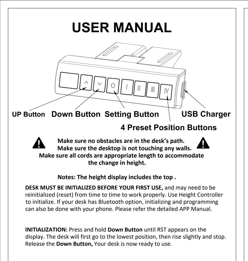
**RESET:** Please note that desk needs to be reset from time to time when it is not working properly in events like sudden power outage and etc. The reset process is the same as initialization and requires more than a simple power-off and power-on for most electronic devices. Unplug the power cord for 20 seconds, plug back in and follow initialization procedure.
