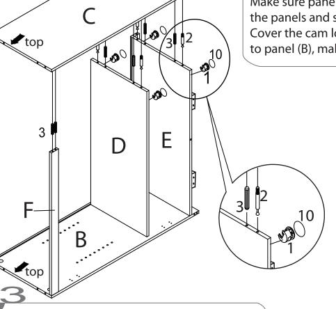
Attach the cam bolts (2) and the wood dowels (3) on panels (C) in the areas illustrated. Then insert the cam locks (1) into panels (D) and (E) with the arrows on the cam locks facing the holes to the side of the panels (D & E). Attach the panels and secure the cam locks, turning clockwise to lock. Cover the cam locks with the adhesive covers (10).
