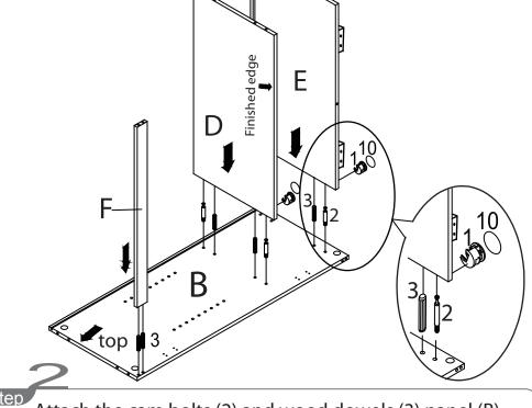
Attach the cam bolts (2) and wood dowels (3) panel (B) as illustrated. Insert cam locks (1) into panel (D) & (E) with arrows on cam locks facing the holes to the side of the panels.
