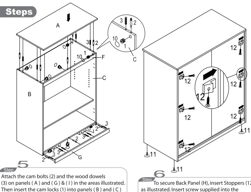
To secure Back Panel (H), insert Stoppers (12) as illustrated. Insert screw supplied into the stopper and slowly tighthen it. Attach adjustable glides (11) to the bottom of the cabinet.
