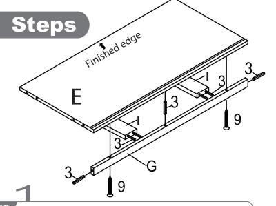
Attached bottom trim back (G) to Bottom board (E) and Base Rail (I) with wood dowel (3) and screws (9) supplied. Insert the wood dowels (3) into the holes on the Bottom trim (G).
