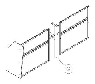
Remove a Side and attach the post  $\bigcirc$  with screws  $\bigcirc$  with help of allen wrench  $\bigcirc$  on the structure.
