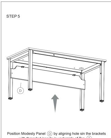
with threaded inserts in underside of Top (A).
