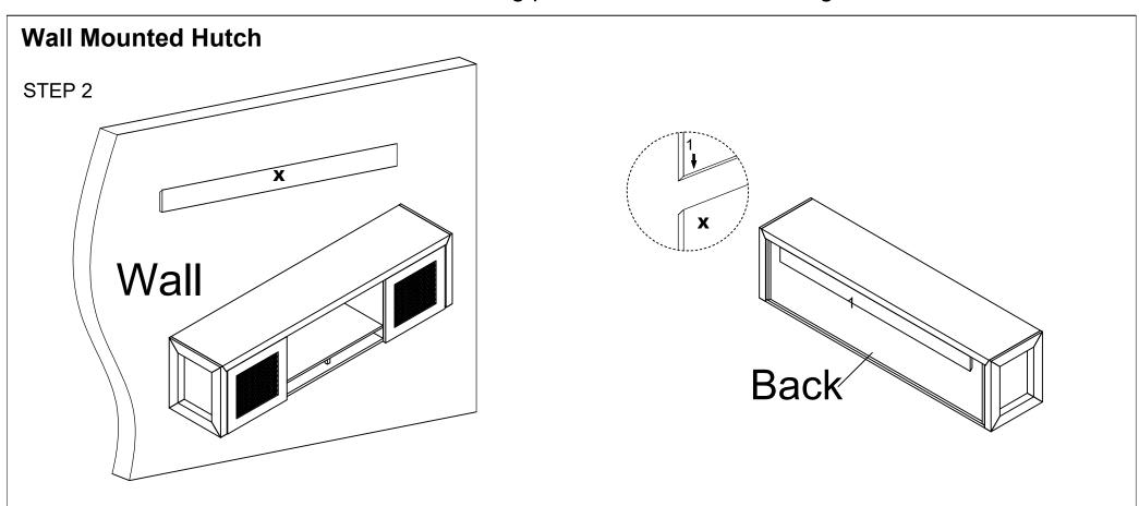
Mounting Board Installation - Due to the various wall construction methods, it is up to a professional installer to secure the Wall Mounting Board to the wall with the proper fasteners and/or anchors as required by the wall construction at the desired mounting location. NBF does not take responsibility for safe, proper fastening.
