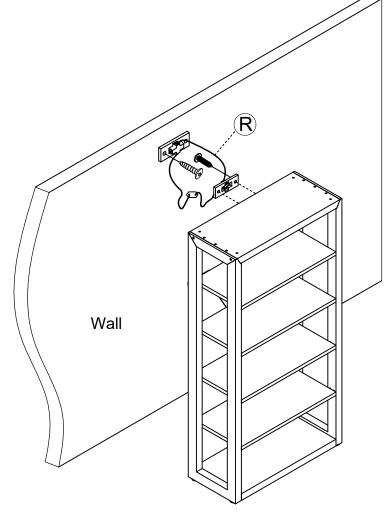
Due to the various wall construction methods, It is up to a professional installer to secure ANTI-TILT SYSTEM to the wall with the proper fasteners and/or anchors as required by the wall construction at the desired mounting location.
