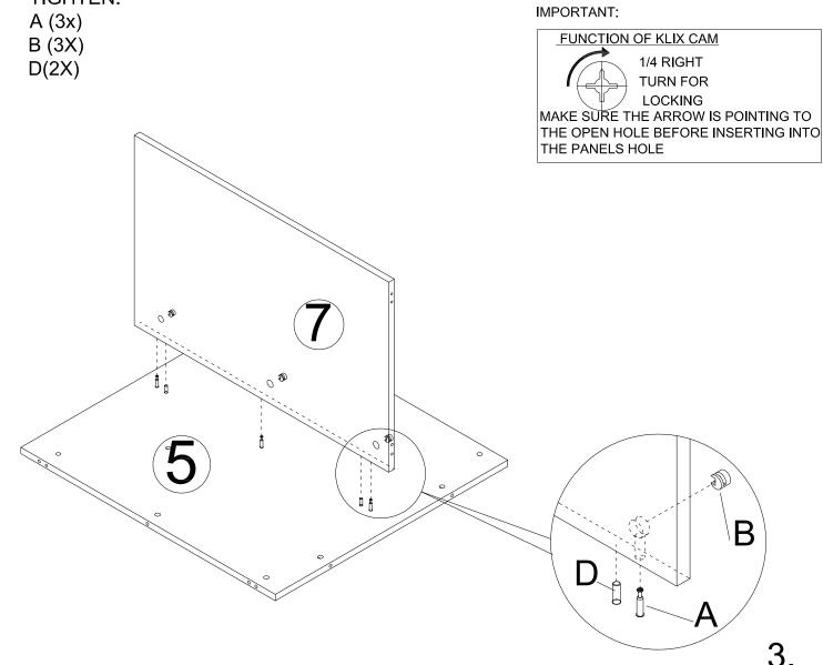
3. INSTALL "A" CAM SCREWS AND "D" DOWELS ON SIDE PANELS 2 . INSTALL "B" KLIX CAMS INTO BACK PANEL ⑤. THEN CONNECT②TO ⑤, TIGHTEN. DO THE SAME STEP TO CONNECT ③ TO ⑤.
