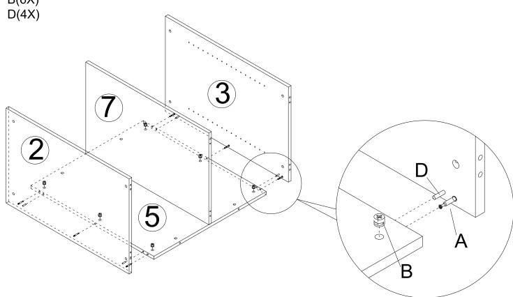
4 INSTALL "A" CAM SCREWS AND "D" DOWELS ON ON BOTTOM PANEL 4. INSTALL "B" KLIX CAMS ON PANEL (2) (3) (5) (7) . THEN CONNECT (4) TO (2) (3) (5) 7, TIGHTEN. REPEAT STEP TO CONNECT 1 TO 2 3 5 7.
