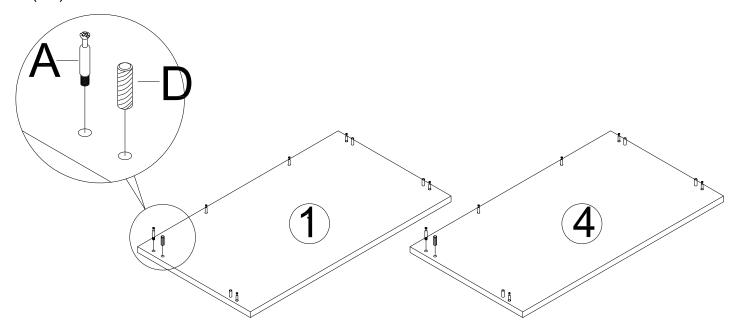
4. INSTALL "B" KLIX CAMS INTO SIDE PANELS ② ③ & ⑤. THEN CONNECT BOTTOM PANEL ④ TO ② ③ & ⑤. TIGHTEN. REPEAT STEP TO CONNECT TOP
