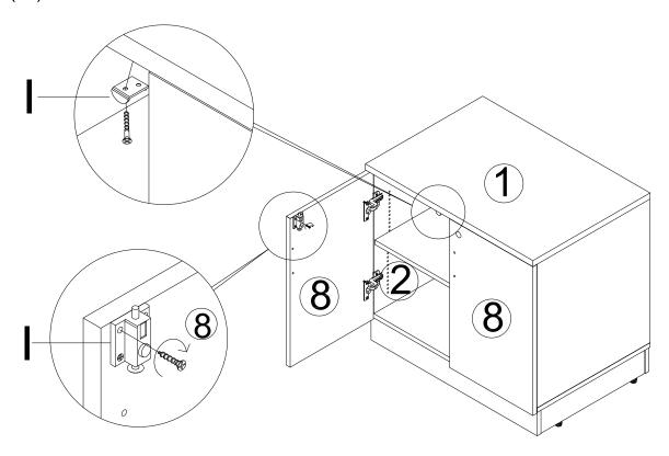
10. INSTALL "H" LOCK UNDER TOP ① & ON INSIDE OF RIGHT FACING DOOR ⑧.( DOOR ATTACHED TO PANEL③)
