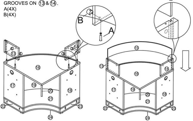
6. INSTALL "A" CAM SCREWS ON THE UNDERSIDE OF COUNTER TOP ② . INSTALL "B" KLIX CAMS ON SUPPORTS ③ AND ④. CONNECT ② TO ① AND ① USING INSTALLED CAM SCREWS AND KLIX CAMS. TIGHTEN. A(4X)
