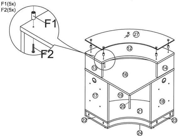
8. USE "C" CAM COVER STICKERS TO COVER ALL EXPOSED KLIX CAMS ON ALL COMPONENTS.
