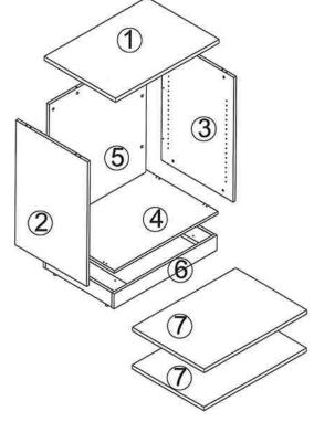
1. INSTALL THE "E" LEVELERS ON THE BOTTOM OF BASE SUPPORT 6. E(4x)
