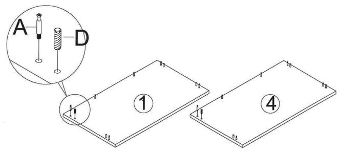
4. INSTALL "B" KLIX CAMS INTO SIDE PANELS ② ③ & ⑤. THEN CONNECT BOTTOM PANEL ④ TO ② ③ & ⑤. TIGHTEN. REPEAT STEP TO CONNECT TOP PANEL ① TO ② ③ & ⑤ .
