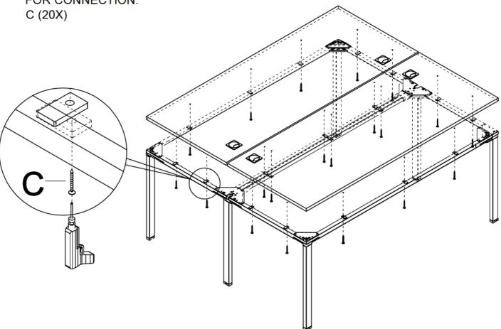
Note: If Installing Desktop divider, Install one desktop first, then see divider instructions before attaching second desktop.
