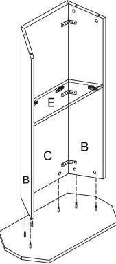
Insert 6 cam locks (H1) into cam lock holes in Panel (B) and Panel (C), use a phillips screw driver to rotate cam locks clockwise to secure cam posts.
