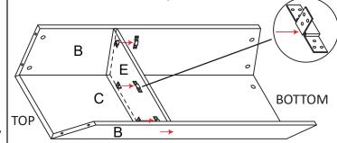
With the shelf assembled, one person can hold the side panels and back panel while another person fix all angle brackets (H4) at the inner edges by tightening wood screws into the pre-drilled holes in
