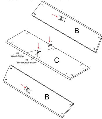
Fix 4 shelf brackets (H6) to the bottom of the shelf panel (E) by screwing wood screws (H3) into pre-drilled holes.
