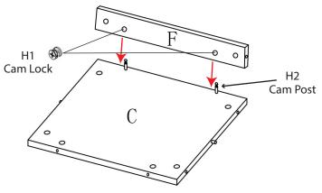
How to join 2 boards with CAM lock:
