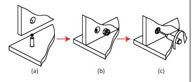
2. Screw 4 cam posts into the holes in Panel D. Attach Panel A and assembled Panel C to Panel D. Insert 4 cam locks into cam lock holes on Panel A and Panel C, use a phillips screw driver to rotate cam locks
