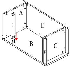
5. Insert 11 cam posts into another Panel B. Install Swing Door g onto assembled panels with sign facing outside, and hold it at its place. Attach the 2nd Panel B to the assembled receptacle body by inserting the cam posts into corresponding holes, then insert and tighten cam locks.
