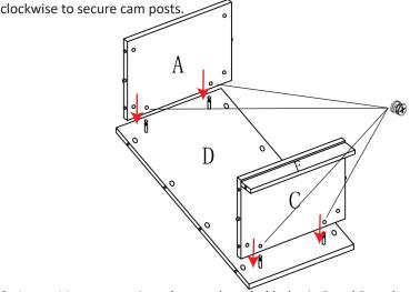
3. Insert 11 cam posts into the pre-threaded holes in Panel B as shown below. Attach the assembled panels in STEP 2 to Panel B and use cam locks to securely lock it in place.
