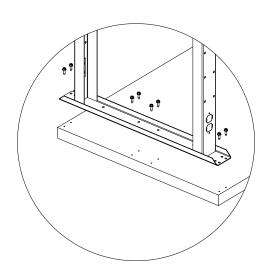
**3.** Place the other adjustable leg on the opposite end of the bench top, using the same procedure shown in step 2.
