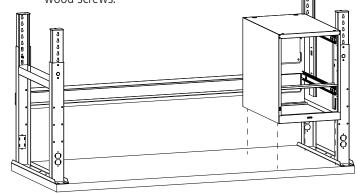
NOTE: After marking where the holes need to be, move the drawer housing to the side before drilling.
