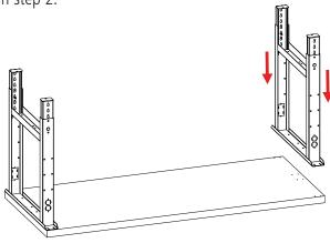
**4.** Attach the stringer (Ref. No. 1) to the rear legs, skipping the top two holes and using the next four holes from the top of each leg. (The legs are symmetrical, so front and rear of the bench will be determined by where youplace the stringer.) Attach the stringer with four 1/4"-20 x 5/8" bolts, lockwashers, and nuts (Ref. No's. 8, 9, 10) on each side.
