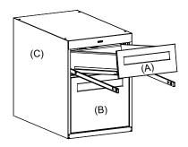
2. Using the housing as a template, mark locations of the holes for the wood screws onto the underside of the wood top. (Recommendation is ½" offset from front of wood top.) Next, drill four holes ½" to ¾" deep into the wood top using a 5/32" drill bit. Once you're finished, secure the housing to the top using four #14-3¼" hex head slotted wood screws.
