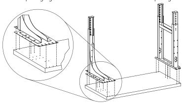
**2.** Turn the table over and line up with the already assembled workstation to create an "L" shape. Once the tables are together, drill four holes through the plate under the assembled workstation and secure with four #14-3/4" wood screws.
