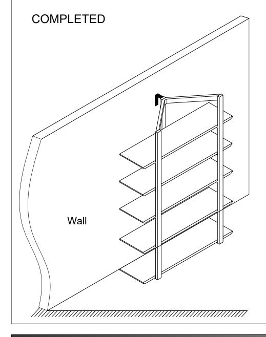
Due to the various wall construction methods, It is up to a professional installer to secure the Nylon Tape(M) Bracket to the wall with the proper fasteners and/or anchors as required by the wall construction at the desired mounting location.
