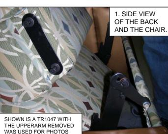
3. SLIDE LOWER BACK BOLT DOWN UNTIL LOWER BOLT IS RESTING IN THE NOTCH AT THE BOTTOM OF THE BRACKET
