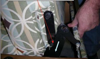
4. ROTATE BACK SO THAT UPPER BOLT RESTS IN THE UPPER NOTCH ON THE BRACKET.
