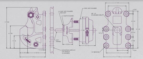
Pushrod length is 3 5/8 in. 92 mm) plus thickness of mounting structure for standard installations as illustrated.
